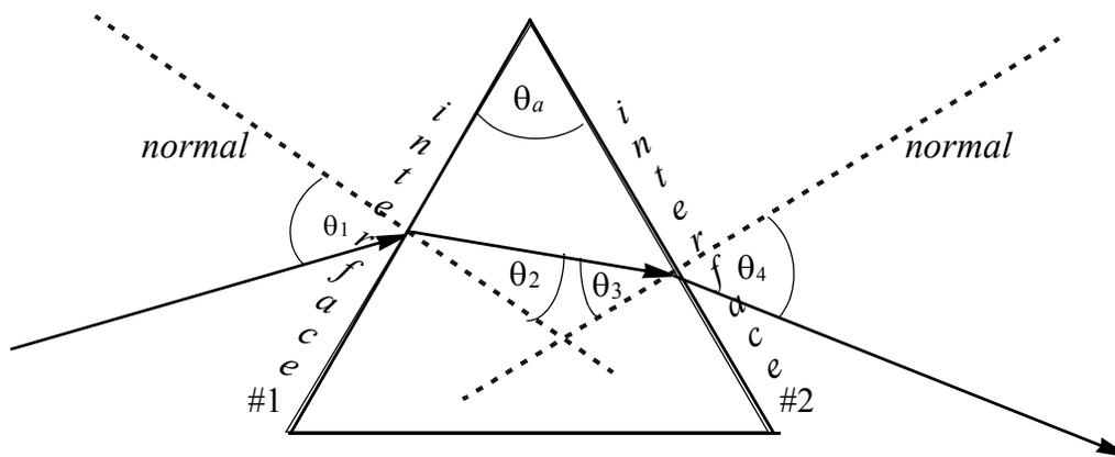
Fig (3) The Two Interfaces of a Prism
