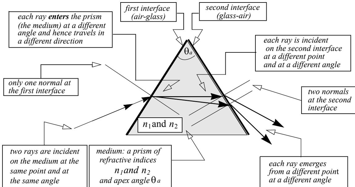
Fig (1) Anatomy of Dispersion of Two Rays of Different Frequencies, Effected by a Prism
