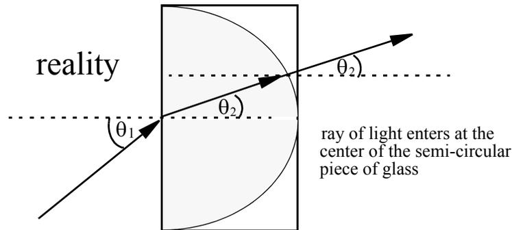
Fig (8) A glass Block with Only One Interface
