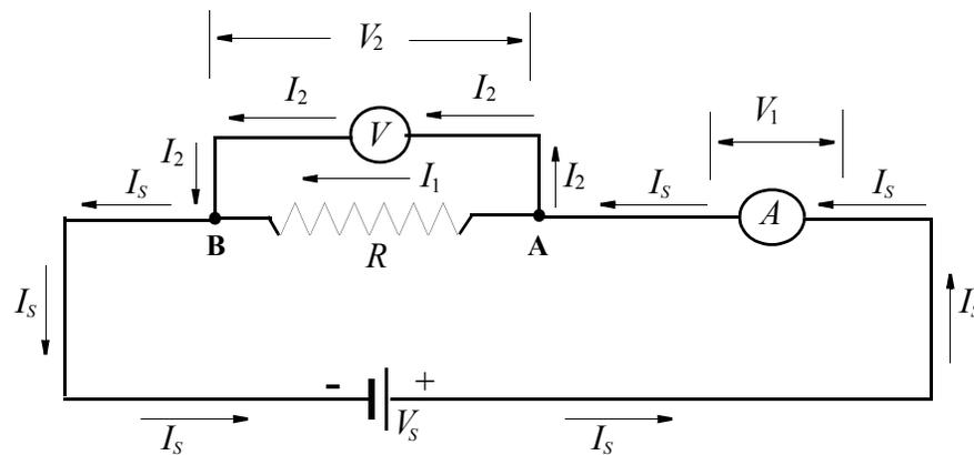
Fig (1) Resistance Measurement using Meters; Configuration #1
