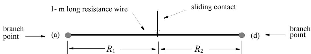
Fig (4) Two Resistances Varied Simultaneously by One Control Knob
