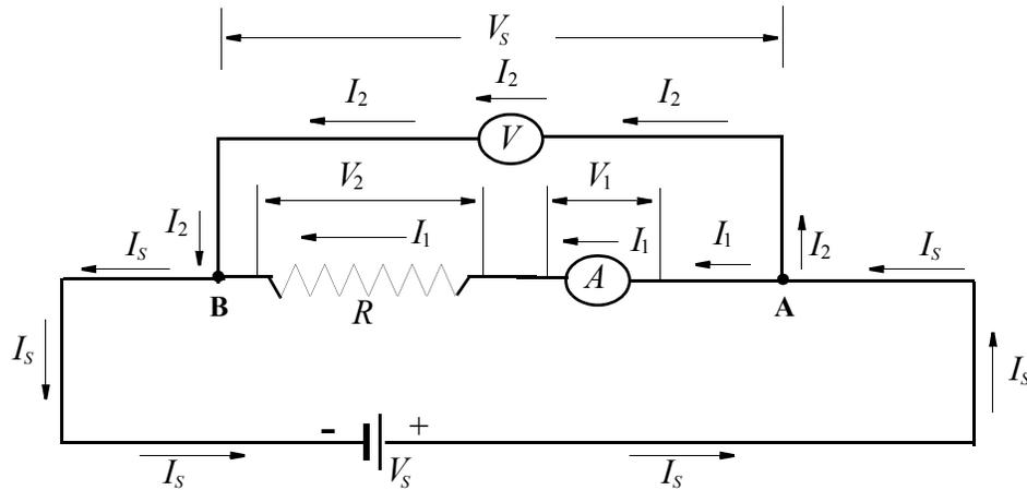
Fig (2) Resistance Measurement Using Meters; Configuration #2
