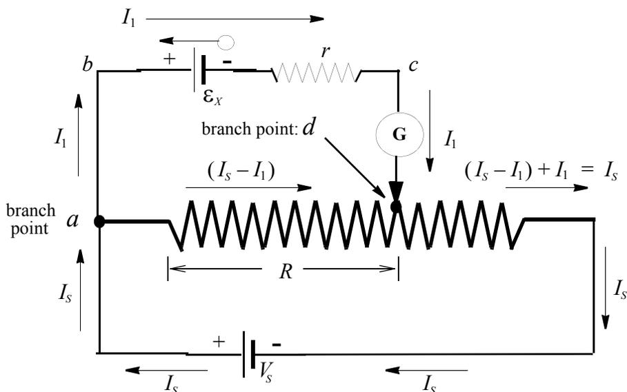
Fig (2) Determination of "emf" of a Battery Using a Potentiometer
