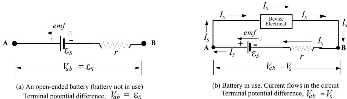
Fig (1) A battery: (a) not in use (b) in use
