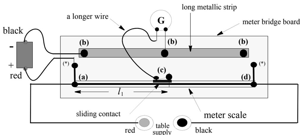
Fig (3) The Potentiometer Circuit
