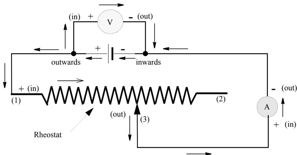
Fig (4) A circuit for Determining the Three Parameters of a Battery
