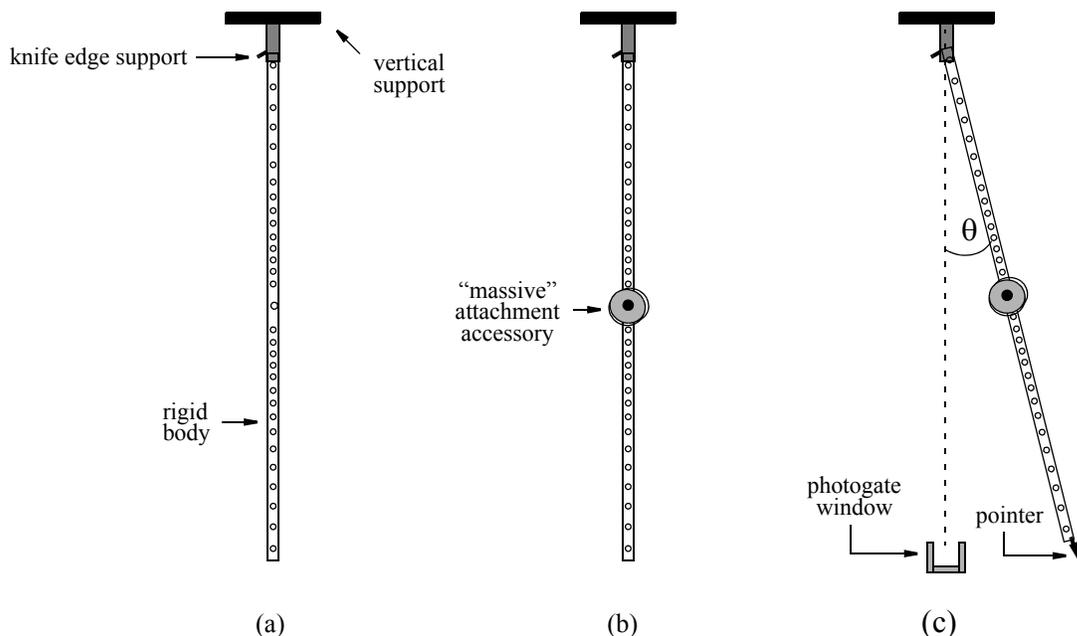
Fig (4) Physical Pendulum
