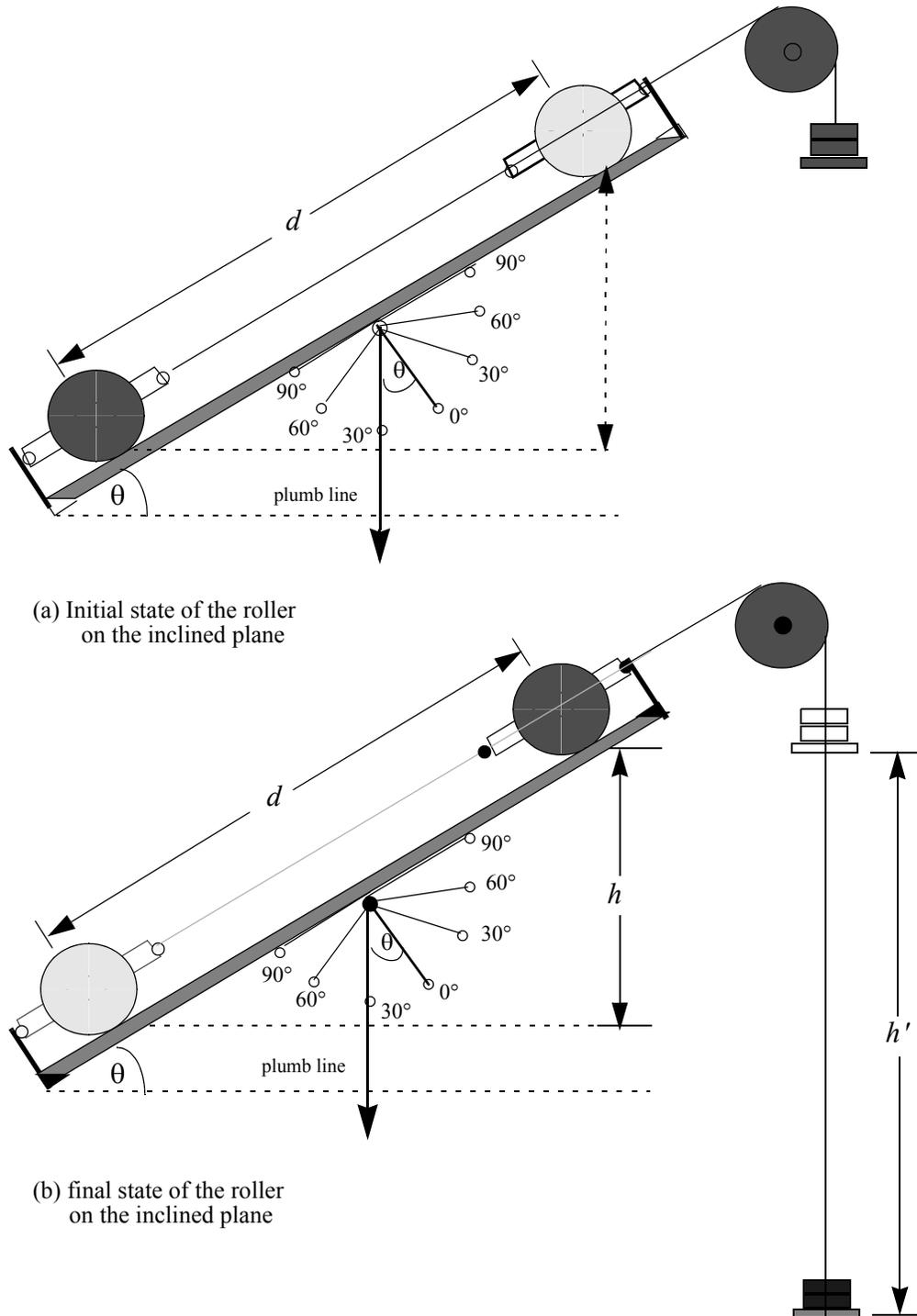
Fig (2) A Roller on an Inclined Plane
