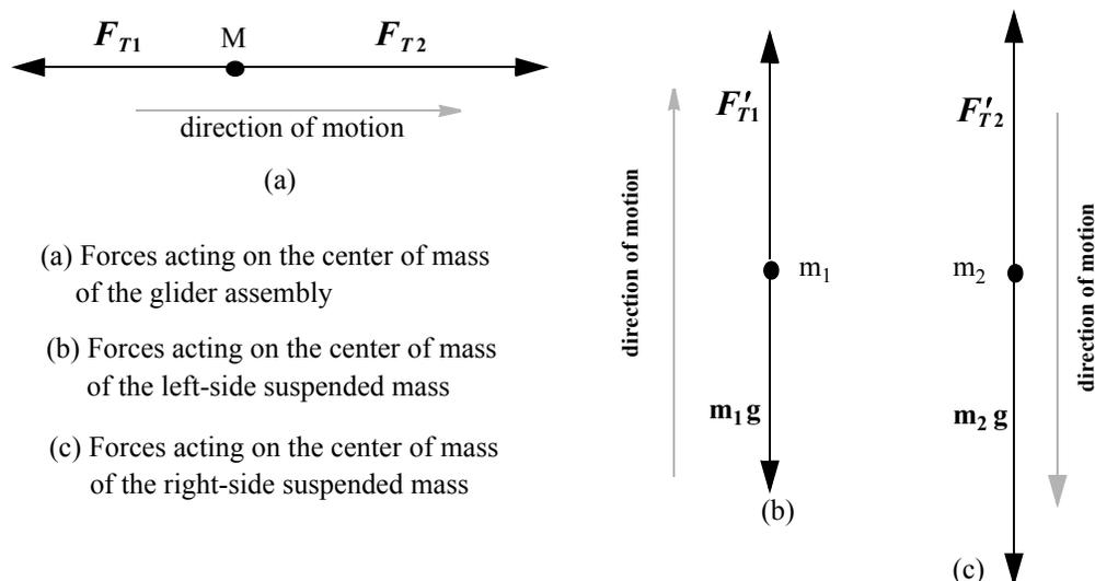
Fig (3) The Force Diagrams
