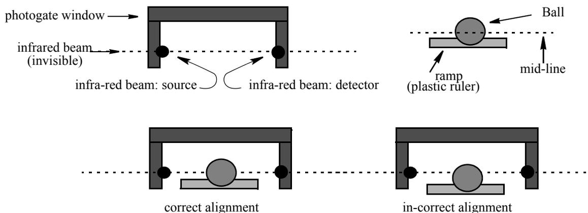
Fig (1) Aligning the Infra-red Beam
